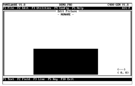
The size of the rectangle corresponds to the selected display type (in this case, display type LCD 8x40 is shown); i.e., the rectangle consists of 8 lines and 40 columns (characters per line). Text or fields can be inserted into the rectangle.
